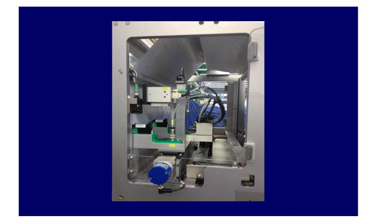
The Print Inspection **SIGNUM HR** is a highly efficient greyscale vision system and the complete solution for 100% optical inspection of print including characters (OCR) on packaging materials during the packaging process. It offers recognition capacity, operating features and operator comfort that exceeds that of most other vision systems. The high reading speed, integrated illumination and outstanding software make the system the best of its kind.
