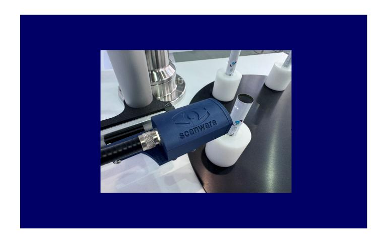
SIGNUM 1DC is a group of code readers designed for use on curved objects such as tubes. A code reader is installed between tube feeding and filling and inspects the print of barcodes or printer marks to ascertain that only correctly labelled tubes are filled, avoiding wastage.
