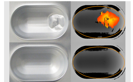
Photo and evaluation view of blister inspection
