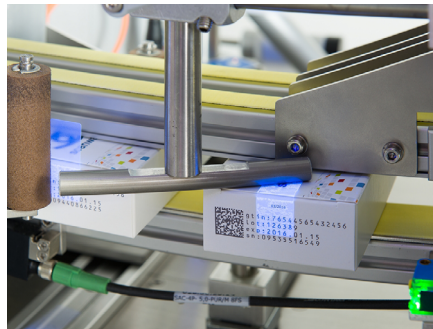
High precision of label placement thanks to precise folding box guidance
